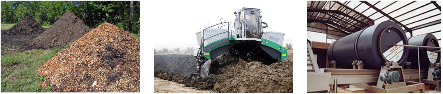
Figure 1: Examples of compost technologies. Static piles (left), windrow facility being turned by a compost turner (middle), rotating drum in-vessel composter (right).
